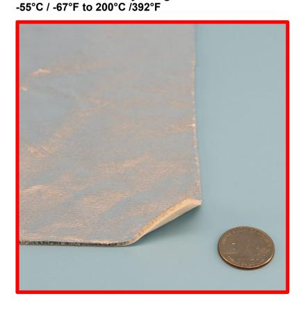
This product is a soft low density silicone foam that has been bonded to an aluminized fabric.
