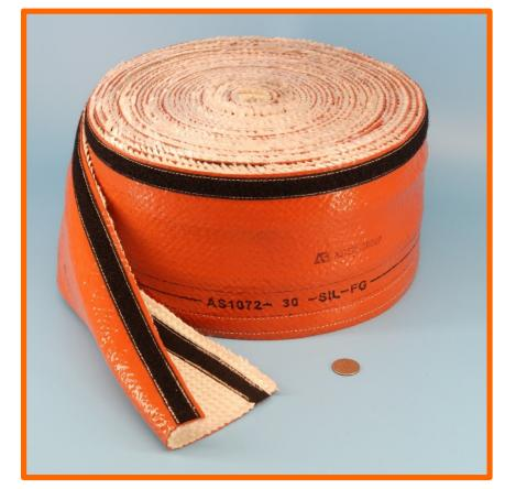
ZeusGard<sup>™</sup> Firesleeve is a high temperature sleeve with YKK brand flame retardant hook and loop or VELCRO<sup>®</sup> Brand closure. SAE AS1072 firesleeve is used for construction of this retrofit sleeve which can be installed without disconnecting hoses, cables or wiring.
