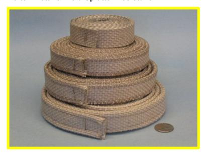
An alternative to asbestos and ceramic based textiles. Highly flexible and minimal shrinkage. High abrasion resistance and tensile strength. Melts above 3000°F / 1648°C. Available with a PSA (pressure sensitive adhesive) to facilitate easy installation (\*see note).
