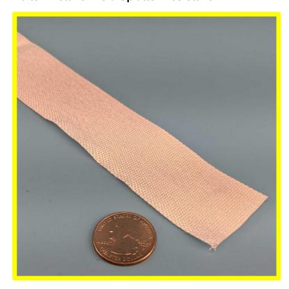
This is a tight weave plain tape in a special thin configuration of 0.015" / 0.381mm thickness.
